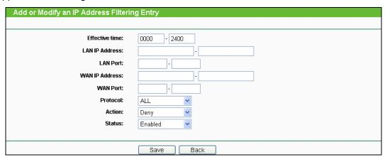
Figure 4-40 Add or Modify an IP Address Filtering Entry
