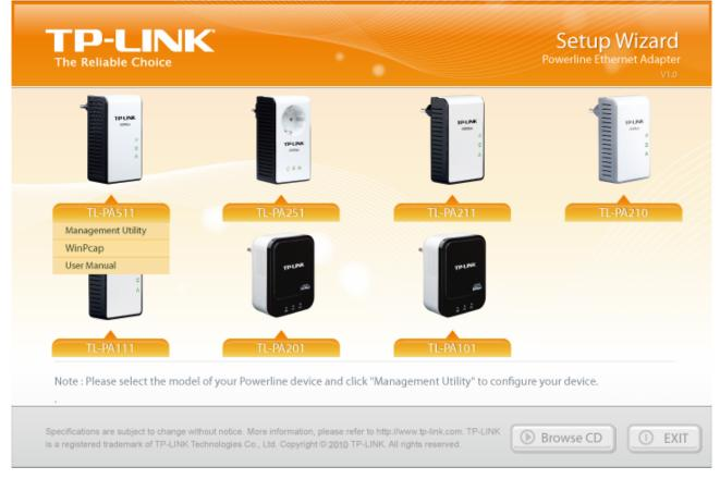
Step 2: Click **Management Utility** and the program installation process will carry out and copy all the necessary files to your system. Follow the instruction step by step to finish the installation.
