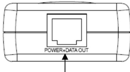
**POWER+DATA OUT:** Connect to the PD or PoE Receiver Adapter with a CAT5 UTP cable.
