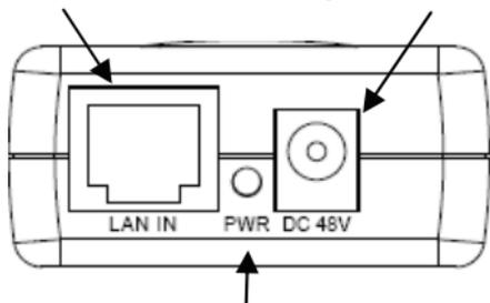
**PWR:** Power LED, a steady green light indicates that the PoE system has detected the PD or PoE Receiver Adapter and the power adapter is working properly.
