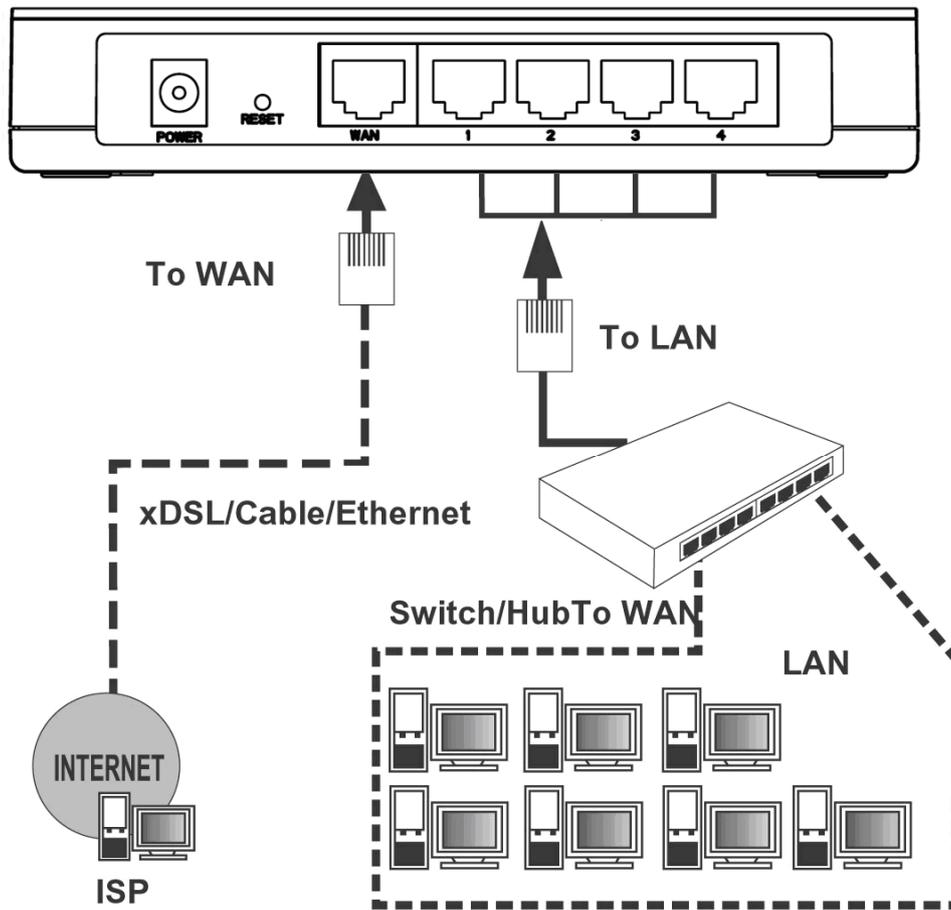
Figure 2-1 Hardware Installation of the TL-R402M Cable/DSL Router
