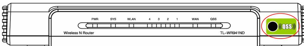
Step 2: Press and hold the QSS button of the adapter directly for 2 or 3 seconds.
