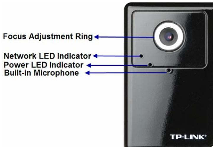
**Focus Adjustment Ring:** Adjust the focus ring to get a clear image.
