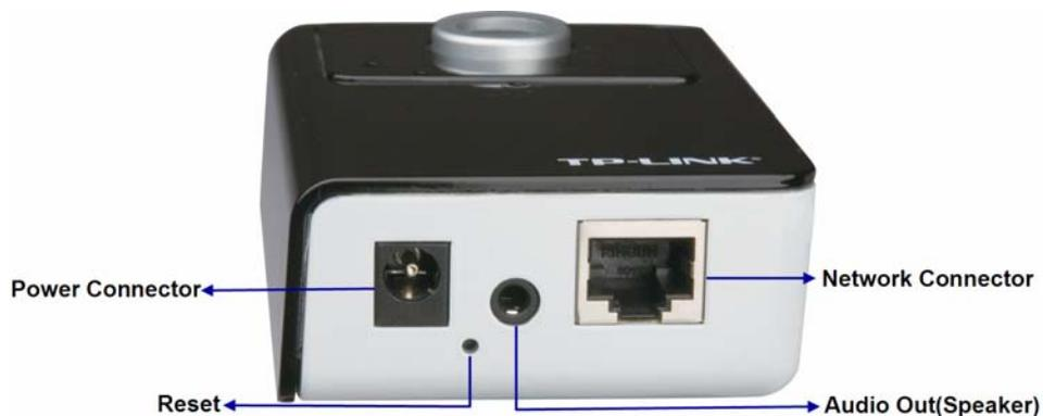
**Power Connector:** The power connector is where you connect the power adapter.
