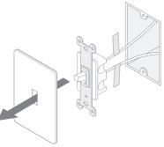
Generally, the **Neutral** wire is white and not connected to the dumb switch; the **Line** and **Load** wires are black and connected to the dumb switch; the **Ground** wire is normally green or copper. If you are unsure, consult a qualified electrician.
