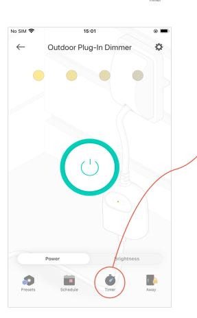
2. Set the time after which the plug-in dimmer will be automatically turned on/off.
