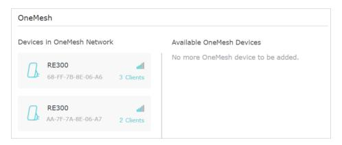
3. Click a OneMesh device to view the device information, or click <number> Clients to view the clients connected to this device.
