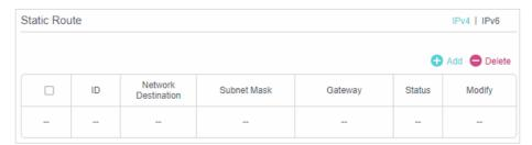
**4.** Click Add to add a new static routing entry. Finish the settings according to the following explanations:
