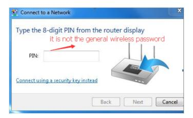
If you cannot find the PIN or PIN failed, you may choose Connecting using a security key instead, and then type in the Network Security Key/Wireless Password;
