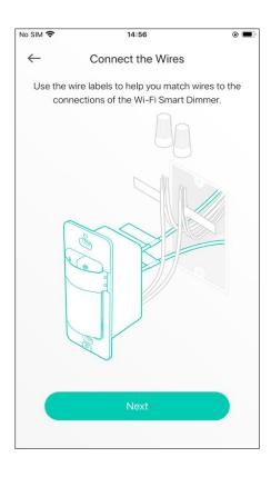
8. Install the dimmer switch and then attach the wallplate.
