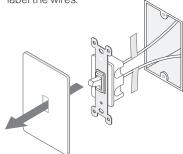
Ground: Usually green or copper. Neutral: Usually white, not connected to the dumb switch.
