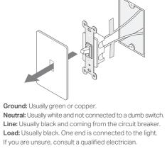
2 Disconnect the wires from the old switch.
