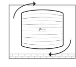
Attach the EAP to the mounting bracket by aligning the arrow mark ▲ on the EAP with the arrow mark ▲ on the mounting bracket, then rotate the EAP until it locks into place, as shown on the left.
