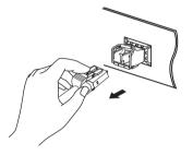
3. Pull the safety latch downwards to release the SFP, and then pull it out
