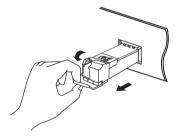
Reinstall the protective dust plug in the SFP's optical bores and place it on antistatic mat or a static shielding bag.
