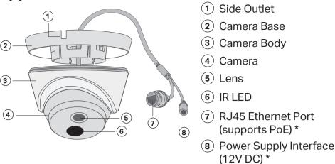
\*The camera's standard power supply is 12V DC or PoE (802.3af/at). The power source should comply with Power Source Class 2 (PS2) or Limited Power Source(LPS) of IEC 62368-1. \*Some models do not have the power supply interface. You can check the detailed specifications on the product page at https://www.tp-link.com/.
