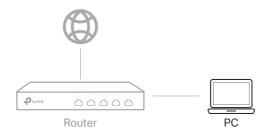
1. Connect a computer to a LAN port of the router with an RJ45 cable properly. If your computer is configured with a fixed IP, change it to **Obtain** an IP address automatically.
