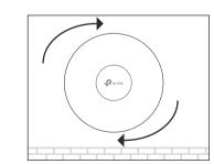
Attach the AP to the mounting bracket by rotating it until it locks into place, as shown on the left.
