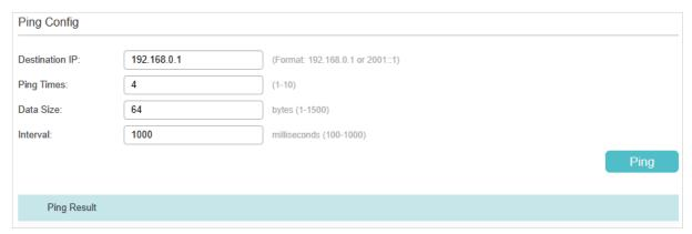
Follow these steps to test the connectivity between the switch and another device in the network:
