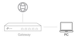
1. Connect a computer to a LAN port of the gateway with an RJ45 cable properly. If your computer is configured with a fixed IP, change it to Obtain an IP address automatically.
