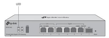
Reset: Press and hold the button for 5 seconds, the SYS LED will flash quickly, indicating the device is being reset to its factory default settings.
