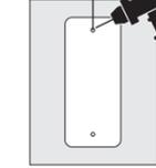
2. Insert two anchors into the holes and use the screws to affix the bracket over the anchors. Starting from the bottom, attach the doorbell to the bracket. Ensure the doorbell is secured to the buckle at the bottom of the bracket.
