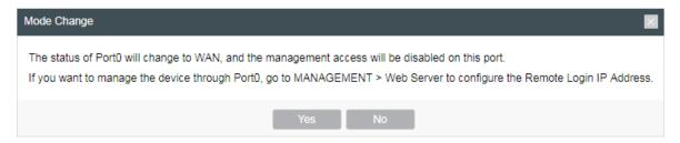
Note that if you select AP Router as the operation mode, the status of Port0 will change to WAN, and the management access will be disabled on this port after the process of quick setup. If you want to manage the device through Port0, configure the Remote Login IP Address. For details, refer to 6.5. Configure Web Server.
