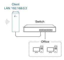
Network requirements: Help the wired devices to connect to the wireless network.
