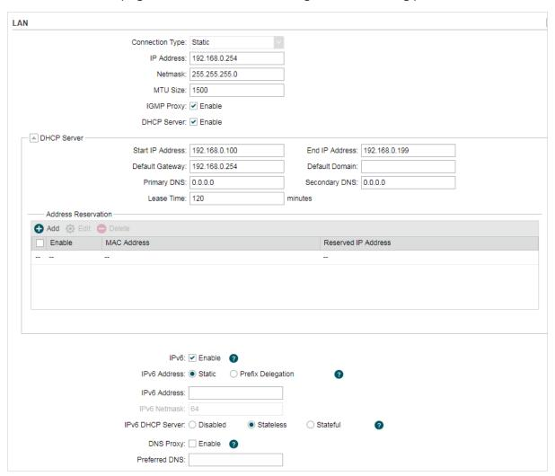
1. For LAN connection type, the device only supports Static.
