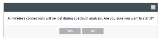
2. Click Start. Observe the curves for a period of time, and then click Stop. The relatively low and continuous part of the average curve indicates less radio noise. Here we take the figure below as an example.
