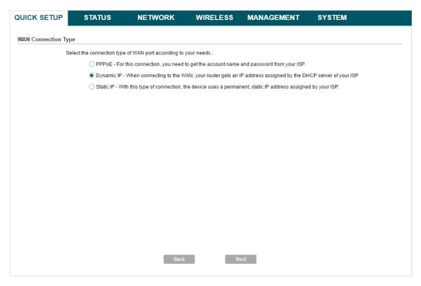
The device supports three types of the WAN connection, including PPPoE, Dynamic IP and Static IP. Contact your ISP to confirm your WAN connection type.
