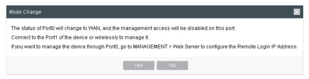
Note that if you select AP Router as the operation mode, the status of Port0 will change to WAN, and the management access will be disabled on this port after the process of quick setup. You can connect to the Port1 of the device or wirelessly to manage it. If your want to manage the device through Port0, configure the Remote Login IP Address. For details, refer to 6.5. Configure Web Server.
