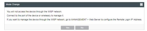
Note that if you select AP Client Router (WISP Client) as the operation mode, you will not access the device through the WISP network after the process of quick setup. You can connect to the port of the device or wirelessly to manage it. If you want to manage the device through the WISP network, configure the Remote Login IP Address. For details, refer to 6.5. Configure Web Server.
