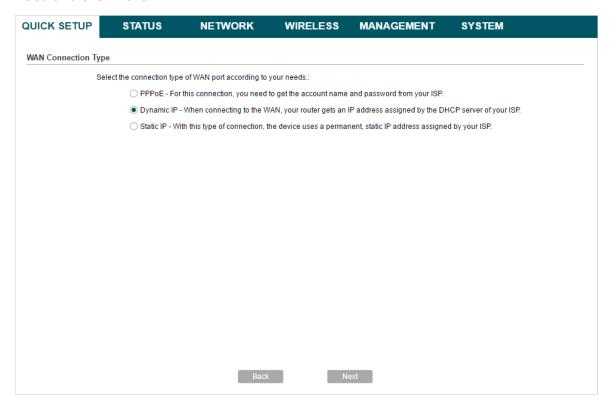
The device supports *PPPoE*, *Dynamic IP* and *Static IP* for the WAN connection. Contact your ISP to confirm your WAN connection type.
