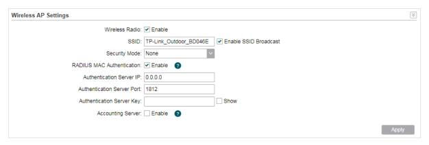
1. Go to the Wireless Page. In the Wireless AP Settings section, specify the SSID.
