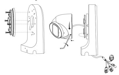
3 Determine routing location for bottom or side exit of cables.
