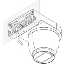
2 Secure the box to the bracket using the screw provided.
