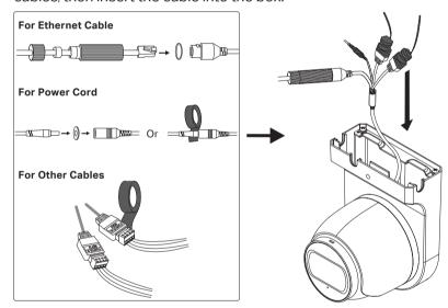
Here we use the side exit for demonstration. After routing the cable, insert the provided silicone plugs to the other two outlets for waterproofing.
