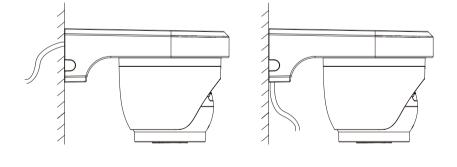
Drill four holes at the marked positions, insert the anchors into the holes, align the bracket to the anchors and drive the self-tapping screws into the anchors through the bracket.
