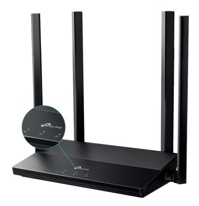
The router's LEDs are located on the front panel. You can check the router's working status by following the LED Explanation table.
