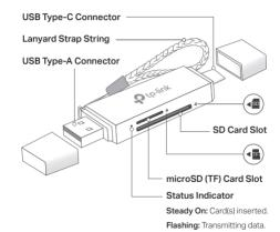
Off: Not connected to the host device yet. No card inserted.
