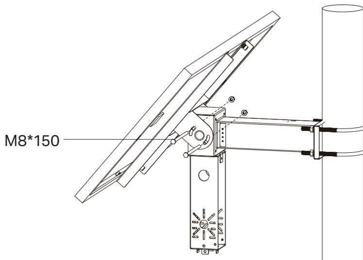
5. Thread the solar panel's four-pin male connector through the side hole of the vertical mount, and connect it to the four-pin female connector of the controller.
