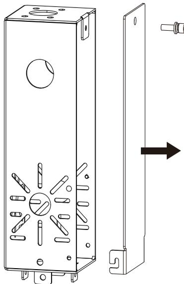
2. Install the vertical mount to cross the horizontal mount, and route the controller's cables through the top hole of the vertical mount.
