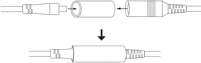
**Note:** For secure waterproofing, you can wrap the connection with over two layers of waterproof tape (not included), as shown below. Wrap the first layer, then cut. Apply a second layer, ensuring no gaps between the connection and tape.
