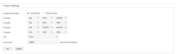
In the Phase-2 Settings section, configure the IKE phase-2 parameters and click OK.
