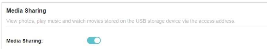
4. When your USB storage device is inserted into the router, your DLNA-supported devices (such as your computer and pad) connected to the router can detect and play the media files on the USB storage devices.
