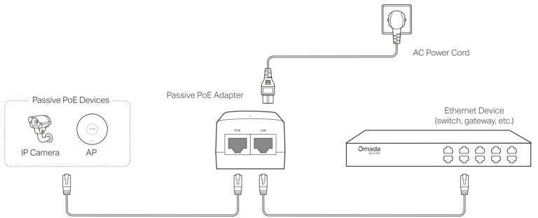
Note: Before connecting a passive PoE device, please check the required voltage in its product manual.
