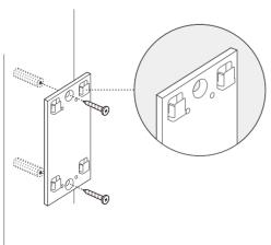
2. Attach the passive PoE adapter to the mounting bracket by sliding the adapter in the direction of the arrows until it locks into place.
