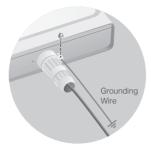
**Note:** For lightning and ESD protection, connect the EAP's grounding terminal to grounding facilities using a proper grounding wire, which should meet local installation requirements.
