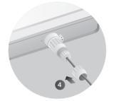
**Note:** To ensure waterproofing, choose the proper seal according to the type and diameter of the Ethernet cable.
