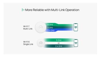
Wi-Fi 6 devices primarily rely on a single link for data transmission. In contrast, Wi-Fi 7 introduces Multi-Link Operation (MLO), enabling devices to utilize multiple links simultaneously, thereby achieving higher throughput, lower latency, and improved reliability.
