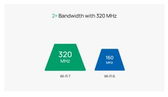
$With 320\,MHz\ ultra-wide\ channels, Wi-Fi\,7\ doubles\ the\ bandwidth\ of\ Wi-Fi\,6's\ 160\ MHz\ and\ the\ number\ of\ subcarriers,\ delivering\ dramatically\ higher\ data\ transfer\ rates.$
