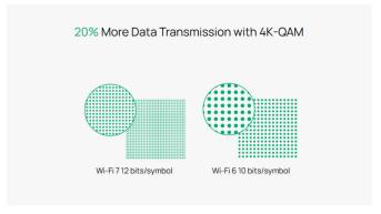
4096-OAM enables each symbol to carry 12 bits instead of 10, increasing theoretical transmission rates by 20% compared to Wi-Fi 6's 1024-OAM. This higher transmission rate boosts data throughput, delivering enhanced speeds and improved network reliability.
